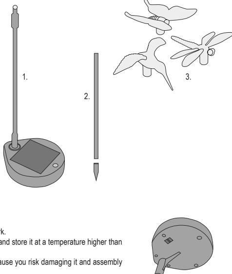
Following the previous operations, the lamp will automatically function, the battery is charged during the day, it switches on in the night twilight and lights continuously. Its duration depends on how long and what light intensity was projected to it before.
