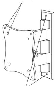
Two drilled holes for wall mounting
