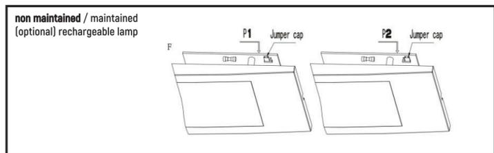
**Non maintained / maintained operation** There is an option to select the non maintained or maintained operation by placing the jumper to the appropriate place according to the graphics sample show.
