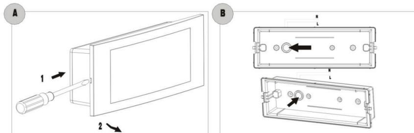
A OPEN THE REFLECTOR AND BASE BY TOOL
