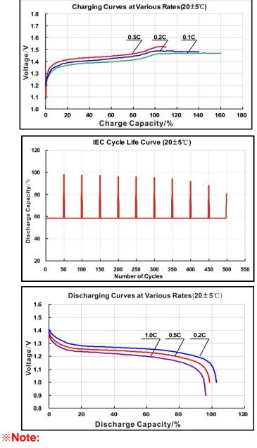
A: Discharge capacity when the battery is discharged at 180mA to the 1.0V end voltage after being charged at 90mA for 16 hours.
